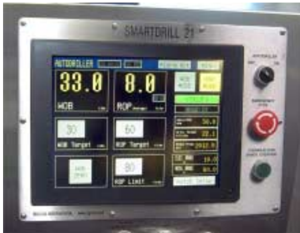
( Driller's Display & Control Panel )
