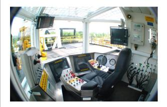
Rigserv Integrated Drilling Controls in a driller's cabin allow the driller to control the drawworks, top-drive, ironroughneck, pipe packer, AC drive, and drilling instrumentation system from an ergonomically designed driller's chair & console.
