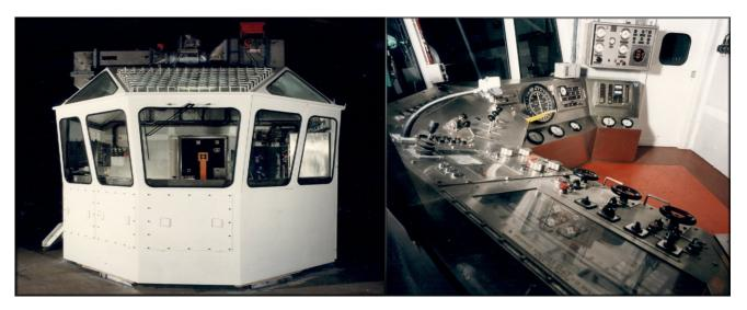
**RIGSERV'S** FIRST INTEGRATED DRILLING CONTROL IN A CABIN ON THE NORTHSEA US\$ 5 BILLION "TOTAL NORTH ALWYN" PROJECT IN 1986.
